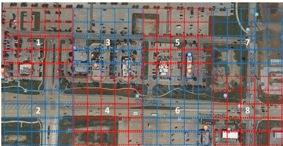
Figure 5: A digital map is divided into equal-sized zones and blocks so that each vehicle is positioned into one zone and detected objects are placed into blocks
